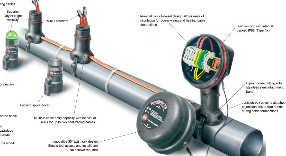
**ZP**...power connection kit is designed for connecting up to three heating cables to power. The heating cable and incoming power are connected in a terminal block utilizing nickel-plated copper terminals to ensure the electrical integrity of the connection over time.
