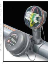
ZL . . . End-of-circuit light kit is designed to provide visual indication of an energized heating circuit. The kit may be utilized as an end termination or a power connection. Electrical connections are made in a terminal block utilizing nickel-plated copper terminals to ensure the electrical integrity of the connection over time.
