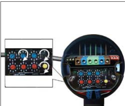
12. Use the rotary switches for settling Control and Limit Temperature, (Celsius or Fahrenheit) and Auto or Manual reset (Control switches on Type "C", Limiter switches on Type "L" and both on Type "CL").
