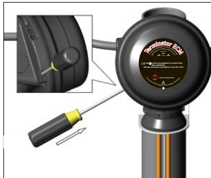
13. Install junction box lid and twist hand tight. Insert screwdriver into ratchet slots located on side of junction box base.
