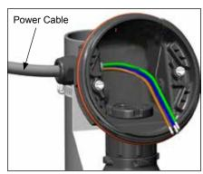
**5.** Install power cable and RTD. Stainless steel RTD tip must extend ≥ 20 mm out of gland.
