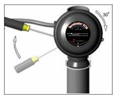
**8.** Use screwdriver to ratchet on junction box lid. Lid will rotate 30 degrees. To remove lid, repeat steps 7 and 8 but in the opposite direction.
