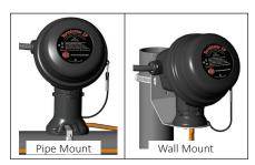
Terminator ZP... is designed to fabricate power connections, in-line/T-splice connections or for making end terminations. The Terminator ZP-XP is suitable for use in hazardous areas (Ex e T6/ T4) harsh industrial environments and has a IP66 rating. The up front positioning of the terminal block permits easy access during termination and for future routine maintenance.
