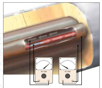
AC voltage will generate a current in the conductor which returns throught the inside surface of the heat tube. There is virtually no measurable voltage on the outer surface of the heat tube, allowing the piping system to be grounded.
