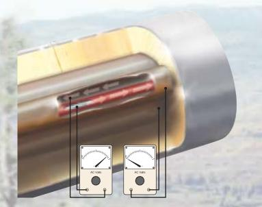
AC voltage will generate a current in the conductor which returns through the inside surface of the heat tube. There is virtually no measurable voltage on the outer surface of the heat tube, allowing the piping system to be grounded.
