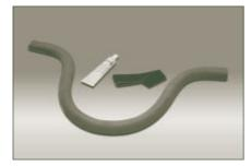
KSR-EJK...expansion joint kits are designed to allow cable to cross a concrete expansion or construction joint. When installed, the kit will allow normal expansion and contraction of the substrate without straining or damaging the heating circuit. Easy-to-use kit includes a reinforced flexible sleeve and RTV adhesive.
