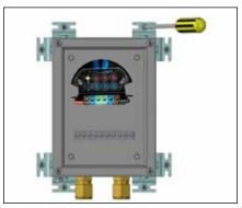
Mounting: Secure wall mount to mounting surface using screws (provided by others).
