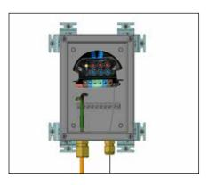
**6.** Terminate cable with appropriate PETK termination kit. Refer to PETK installation instructions. Push excess cable back through gland. Tighten cap securely. Tape cable expansion loop to pipe.
