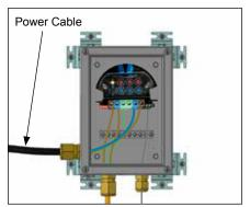
8. Install power cable. Complete system wiring. Terminal set screws shall be tightened to a torque value of 1,4 Nm (12,4 lb-in). See wiring details. Set modules electronic control and/or control limiter at desired setpoints.
