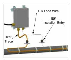
12. Slide IEK insulation entry kit onto RTD lead wire. Fix RTD lead wire and sensor to pipe.
