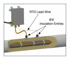
13. Install IEK insulation entry kit to seal heating cable and RTD lead wire penetrations through insulation cladding.
