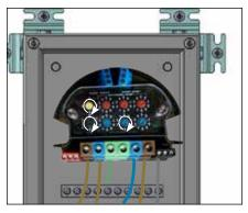
**10.** Use the rotary switches for settling Control and Limit Temperature, (Celsius or Fahrenheit) and Auto or Manual reset (Control switches on Type "C", Limiter switches on Type "L" and both on Type "CL").
