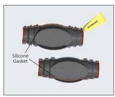
**7.** Install silicone gasket, cutting off excess. Apply RTV sealant to both halves.
