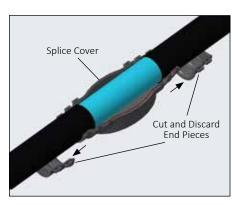
**6.** Cut top and bottom splice cover ends to match outside diameter of tubing bundle.
