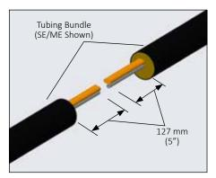
1. Remove outer jacket and insulation from tubing bundle approximately 127 mm (5") from end of the tubing bundle. Where required ensure sufficient heat trace is available for electrical splice. See instructions included with heat trace kit (purchased separately).
