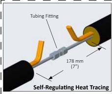
Cut 38 mm (1.5") off the end of the tubing and make tube fitting connections with appropriate fittings, provided by others. If no electrical heat trace is present, go to Step 4.
