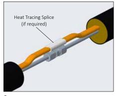
If bundle includes electric heat trace, make-up splice per instruction included with heat trace kit. This should be accomplished after fittings are leak tested.
