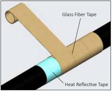
4. Wrap tube and heat trace with 1 pass of reflective tape (25% overlap), then wrap with 3 passes of glass fiber tape (50% overlap), or until fiber tape is equal to original bundle insulation thickness.
