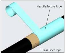
**5.** Complete with additional passes of heat reflective tape.
