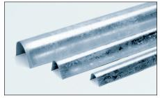
**TFK-4** galvanized steel channel 30 mm x 21 mm (1.18" x .84") covers SnapTrace heat transfer compound applied to 3/8" or 1/2" O.D. tube tracers.
