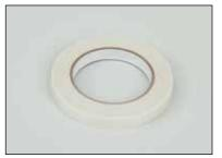
**FT-1H** fixing tape for circumferential banding of SafeTrace tracer to piping every 12" (300 mm) or as required by code or specification. Tape is 1/2" (13 mm) wide x 108' (33 m) long.
