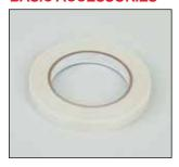
FT-1H fixing tape for circumferential banding of SafeTrace tracer to piping every 300 mm or as required by code or specification. Tape is 13 mm wide x 33 m long.
