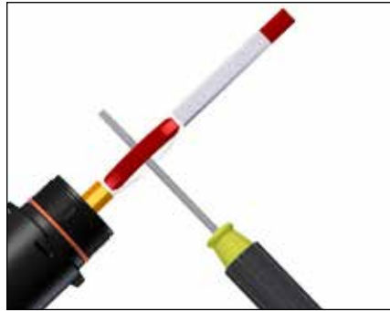
1b. Separate braid strands at edge of overjacket and pull cable through opening in braid.
