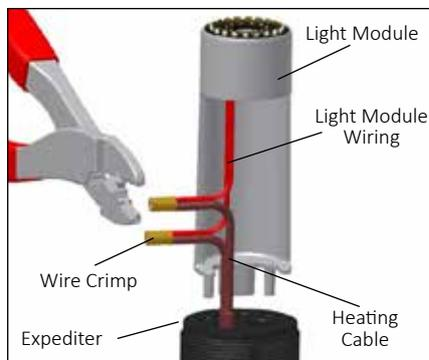
**8. When using crimps:** Connect heating cable to light module wires using small crimps. See steps 8–11.
