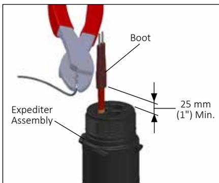
**7.** Terminate cable with appropriate SCKT termination kit. Refer to SCKT installation instructions. Push excess cable back through expediter. Remove braid pigtail. Tape cable expansion loop to pipe.
