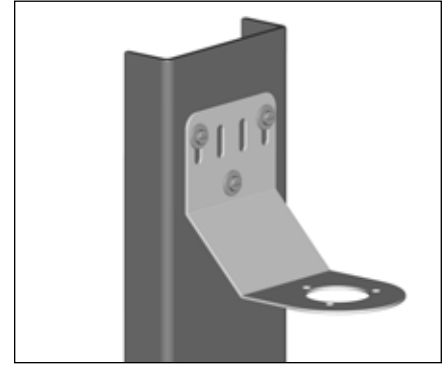
2b. Mounting Method 2: Secure wall mount bracket to mounting surface using customer supplied screws, flat washers, and nuts.
